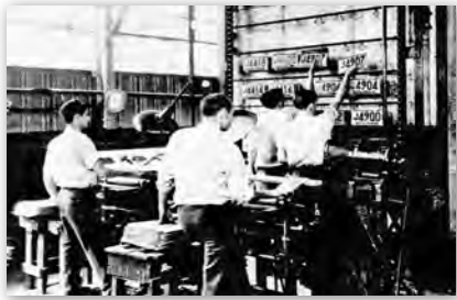
Figure 115. Photograph of inmates manufacturing license plates at Western Penitentiary in 1937. Products made through inmate labor evolved over time at Western Penitentiary. A few handicrafts were made by inmate in their cells, but most products were manufactured in the factory-like setting of the penitentiary's workshops. License plates, made in the Tag Plant (Building 11), were one of the notable goods manufactured on site, as well as metal office furniture and shoes (The Pittsburgh Press, 12/12/1937, p. 9).
