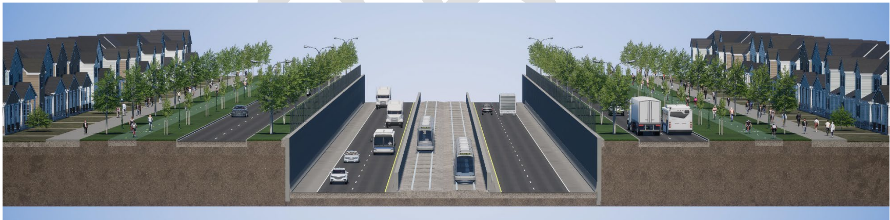
Figure 16. Alternative 3: Partial Cap Section with Subway
