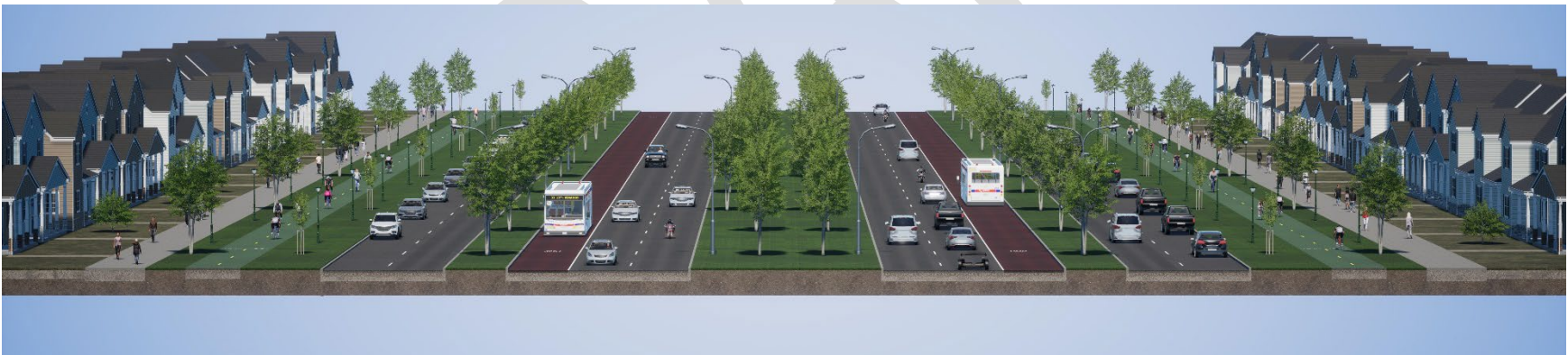
Figure 12. Alternative 2B: Neighborhood Boulevard with BRT in Semi-Exclusive Guideway in Inner Lanes
