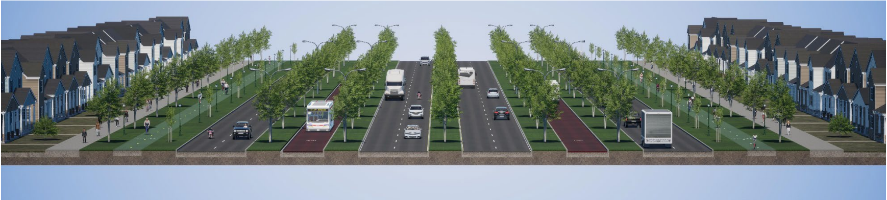
Figure 11: Alternative 1B: At-grade Section in Partially Capped Expressway with BRT in Semi-Exclusive Guideway
