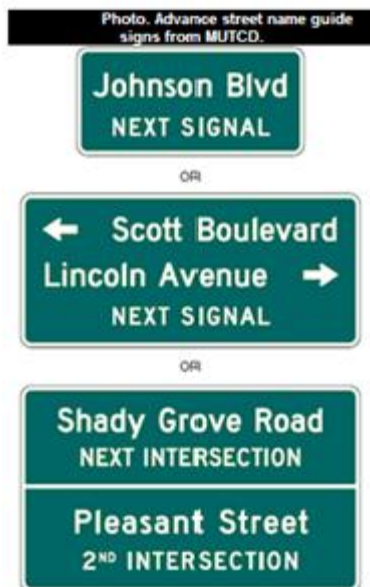
Exhibit 4-33 Advance Street Name Sign
