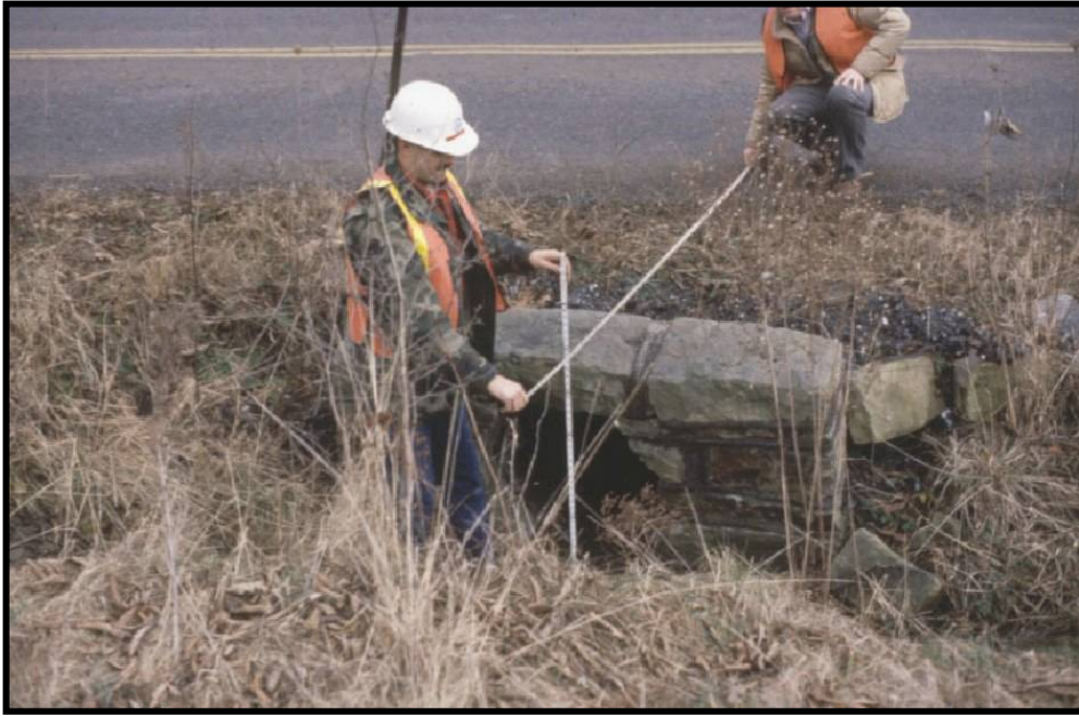
Example of Measuring Invert Depth
