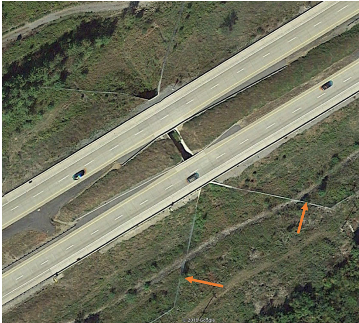
Area View of Wildlife Crossing with Channeling Guide Fence (I-99 PennDOT District 2)
