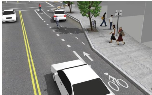
Exhibit 8.6.1 Right-Turn Transition Through Bike Lane
