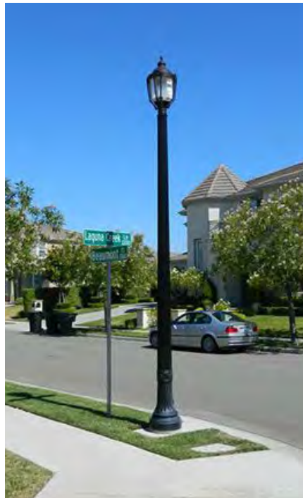
Pedestrian pole with fluted base and lantern fixture
