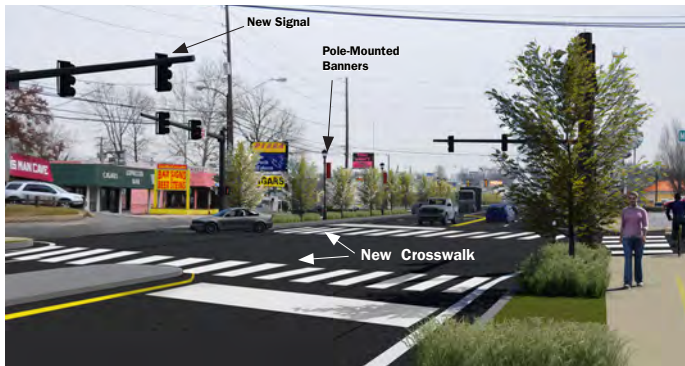
Phase 3: Installation of signal and crosswalks at Millstream Road
