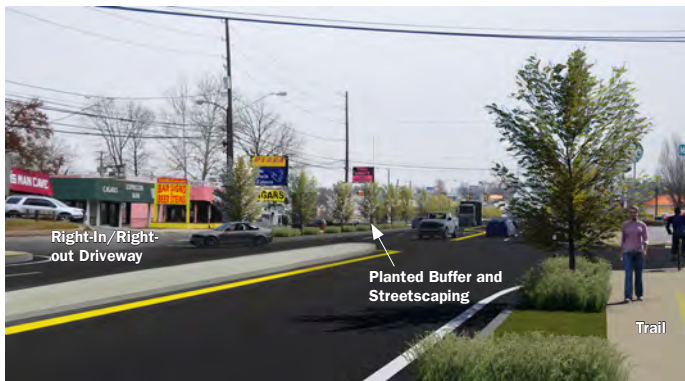
Phase 2: Reconstruction of roadway and installation of multi-use path and streetscaping improvements
