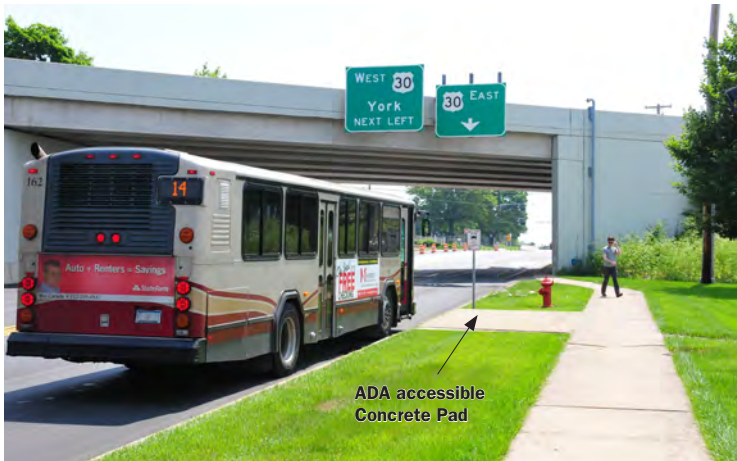
Example of standard bus stop detail
