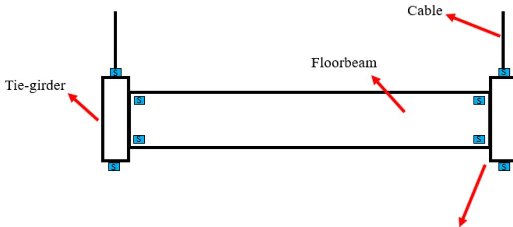
After simulating the corrosion, the stiffness of the boundary condition of floorbeams will be less than the pristine condition. Therefore, less load will be transferred to the East tie-girder.
